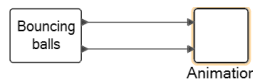
Figure 19.1: The Bouncing balls block output vectors provide the x and y coordinates of the balls.
