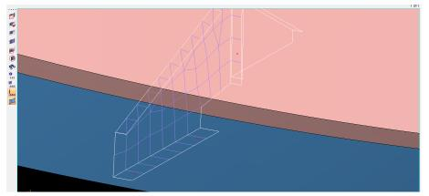
This should allow you to visualize the red points under this mesh, which designate the location of the connectors we want to make.
