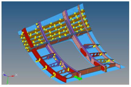
All of the FE for the spot welds has now been deleted, and only the connector entities remain. The connectors should turn from green to yellow.
